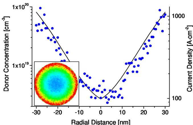
**Figure 1:** Calculated current density (dots) passing through the wire having the dopant concentration (line) calculated from the KPFM data ; the inset shows the calculated current density cross section for this dopant distribution.
